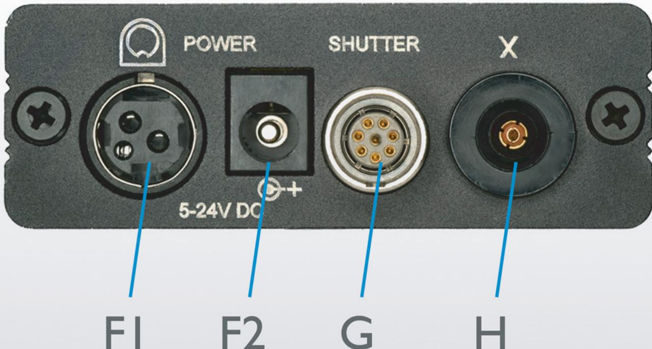
**F1** DIN plug connection for external power supply
